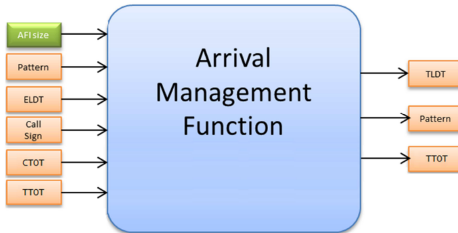
Figure 3: Arrival Management Function - input/output model
